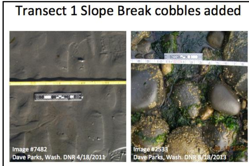
Figure 4: Digital images showing surface sediment expression related to Fig. 10. Image on left is categorized as sand with fines (1) and image on right is cobbles (4), 2.5 years later and 0.5 m higher in elevation.
