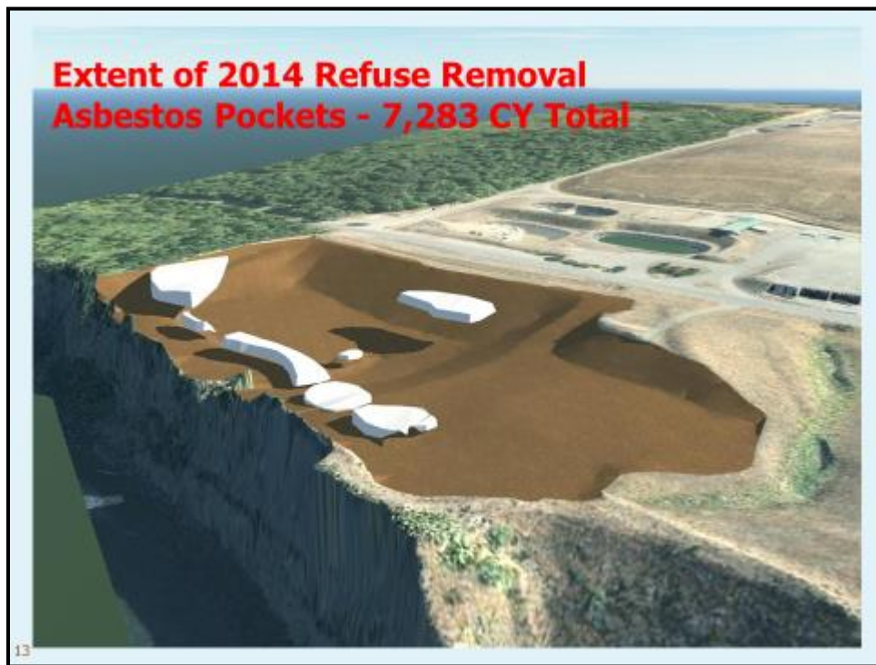
Figure 6: Computer rendition of the extent of the asbestos pockets in the 304 Cells.
